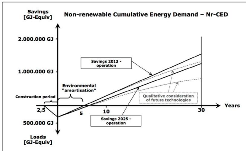
Fig. 4: Environmental effect of the tunnel – Nr-CED.
