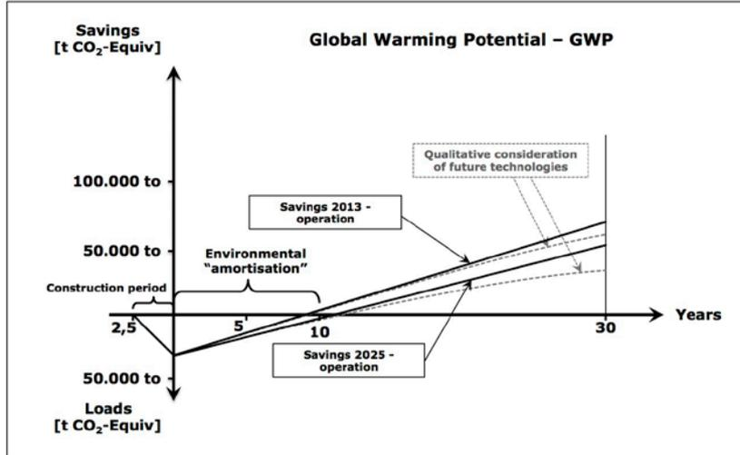
Fig. 2: Environmental effect of the tunnel – GWP
