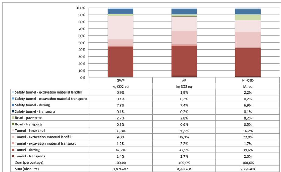
Fig. 1: LCA results tunnel new construction including maintenance.
