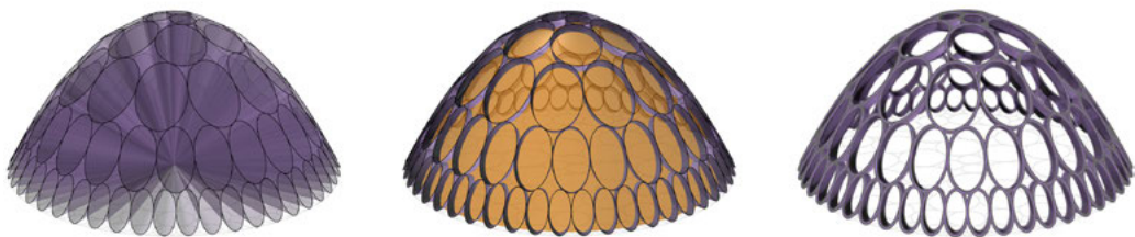
Figure 3. Left: Discretisation of the dome with elliptical rings and generation of the cones by extruding the ellipses to the centre of the base of the dome. Middle: Offset surface to trim the apex. Right: Thickening of the conical rings as an immediate solution to acquire rigidity.
