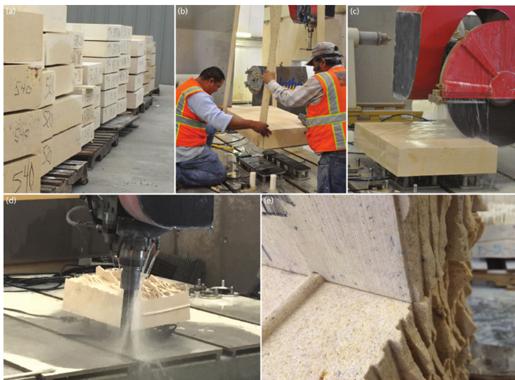
Figure 8. Fabrication process: (a) The stones cut at the bounding boxes of the voussoirs. (b) Placement of the voussoir bounding box cut on the milling bed. (c) Rough cuts with a circular blade to create the intrados. (d) Processing of load-transferring side faces with custom-made tool to create the notch lines. (e) Adjacent stones test-assembled to verify alignment of rough-cut lines.
