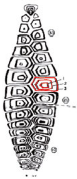
Figure 9a. Diagrammatic representation of plate accretion (left). A row of calcite plates is shown that grow in size while moving towards the middle. The principle of growth is abstracted in the computational design tool (right).
