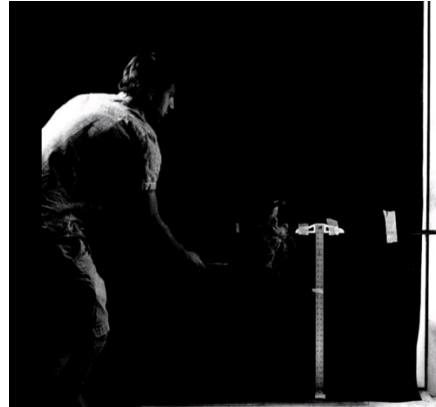
Fig. 9: Smoke tube test of the DSF.
