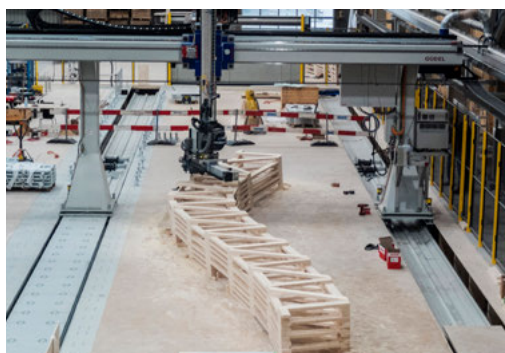
Figure 19. Automated fabrication and assembly using a 6-axis gantry robot (ERNE AG Holzbau) (Willmann et al. 2015).
