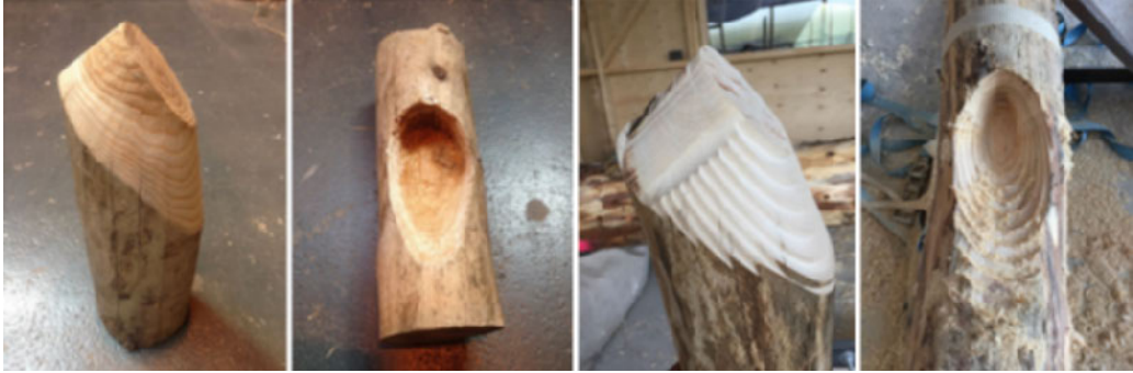
Figure 9. Development of the mortise and tenon connection.
