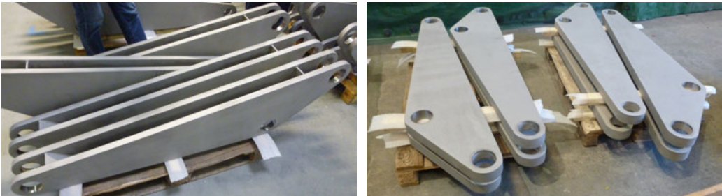
Figure 16. Left: The 2 x 30 mm thick plates. Right: The 60 mm thick plates, which comprise the edge scissors.
