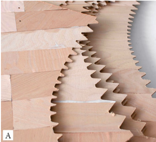
Figure 8a. Multiple plywood strips laminated with different veneer directions to influence their elastic bending behaviour.
