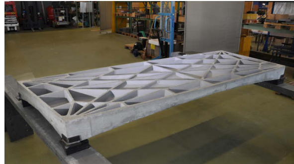
Fig. 3: Integrated funicular floor system [10].
