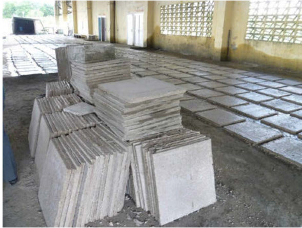
Fig. 4: Prefabricated elements with LC 3 cement produced in Cuba, Siguaney a) hollow concrete blocks b) hydraulic tiles (courtesy of F. Martirena)
