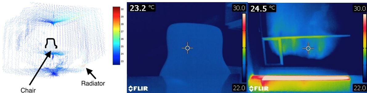
Fig. 6: SMART Sensor point cloud (left) with components shown in comparison to images of the same features from a FLIR E60 (middle and right).
