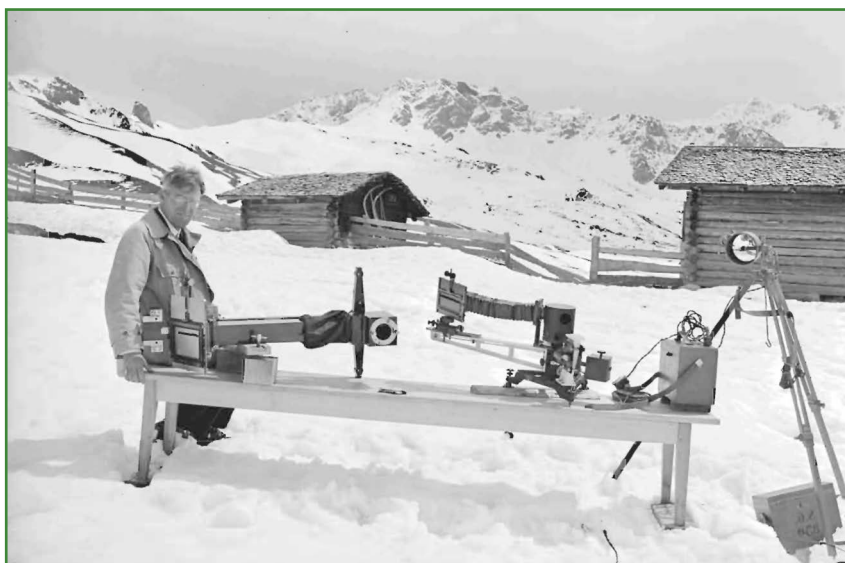
Figure 16.3: Götz (April 30, 1930) and the apparatus used for surface ozone measurements from Tschuggen (Arosa) (see Götz and Ladenburg, 1931).
