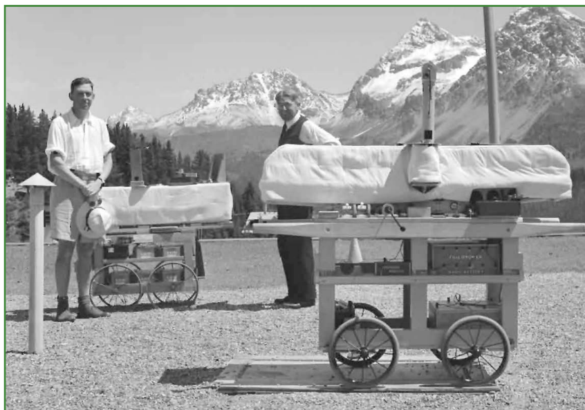
Figure 16.2: Comparison of two Dobson instruments at Arosa on the roof of the Kurhaus Florentinum (1954). On the left: C. D. Walshaw, serving as travelling scientist to check and calibrate the Dobson spectrophotometers. F. W.P. Götz can be seen standing in the centre behind the instruments.
