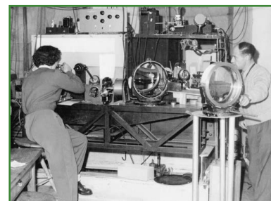
Figure 17.6: Installation of the first infrared spectrograph for the analysis of the solar radiation by the Migeotte Group (Source: HFSJG)
