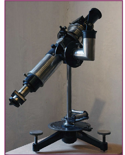
Figure 12.2: Picture of the Weber polarisation-photometer used by Dorno for the measurements of polarisation and intensity at any point of the sky. The vertical tube on the side of the instrument allows direct comparison with the zenith intensity and polarisation, which can then be determined by a Weber photometer in absolute terms.
