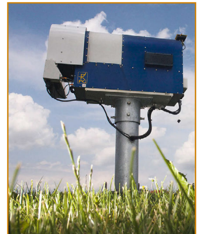
Figure 10.5: Operational microwave radiometer profiler mounted in MeteoSwiss Payerne in 2009 (Calpini et al., 2011) (Source: B. Ruffieux).
