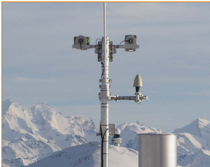
Figure 9.13: External receiver and transponder systems were employed during the accep- tance test periods. The picture shows the test equipment and in the background the weather radar under test (Photo: H. Krähenbühl).
