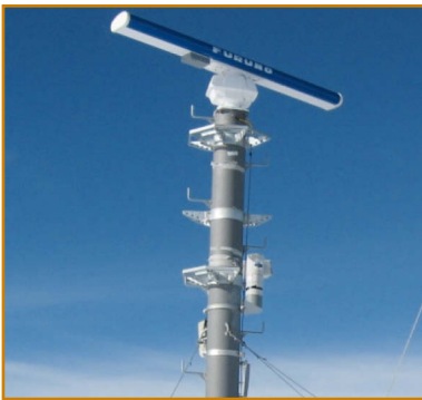
Figure 9.15: X-band weather radar operated by ETH on the summit of the Klein Matterhorn during a research campaign in 2007 and 2011 (Foto: M. Savina).
