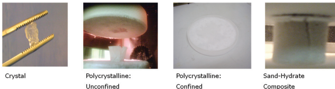
Figure 2: Different forms of THF hydrates synthesized as low pressure analogues.
