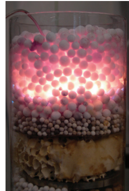
Figure 2: Photograph of diesel flame ( P=4 kW, \phi=2.5 ).
