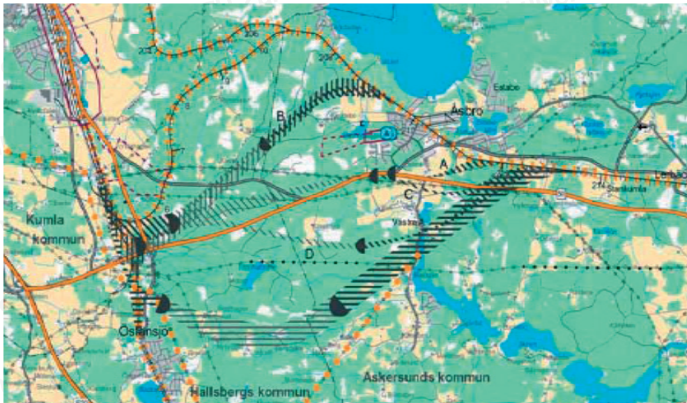
Figure 1: Example of alternative routes (hatched areas) in initial study for a railroad. The project concerns the cargo track via Bergslagen, section Hallsberg – Degerön, County of Örebro.
