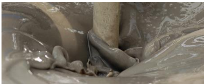
Figure 49: Example of a water-based drilling fluid 18 .
