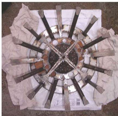
Figure 62: Picture of electro-pulse drilling bits (Bommer, 2012).
